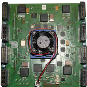
Figure 5. Bottom side of the FEB/D-1024 mother board showing the 8 connectors receiving the cables from the FEMs.
