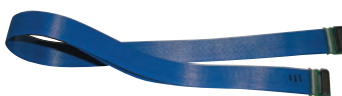
Fig. 3: SAMTEC cable A flat coax cable assembly connects the Front-End Module to the PETsys FEB/D board.
