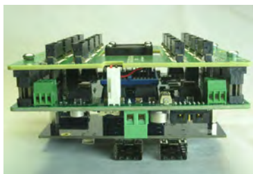
Figure 6. Clock&Trigger module. Bottom view showing the connectors for the 16, 3M 3896 series cables providing clock and trigger signals to the FEB/D modules .
