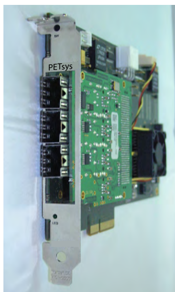
Figure 7. The DAQ board plugs directly into the PCI express bus of the DAQ computer. The three SFP+ connectors on the front panel receive the 3 optical links from the FEB/D chains
