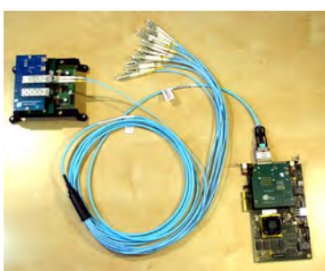
Figure 8. The DAQ board is connected to the FEB/D module using a 12xCXP/SFP+ high-speed optical link .
