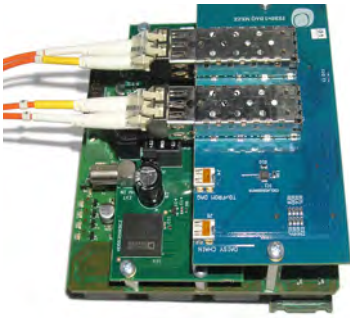
Figure 4. Top side of the FEB/D-1024 module with DAQ mezzanine.
