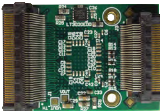
Fig. 2: FEB/A_V2 Top and bottom view. The connector to the right connects to the FEB/S, the connector to the left connects to the FEB/I. The board, including connectors, measures 39x25 mm.
