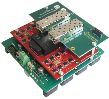
Figure 6: FEB/D-1k unit. Top view of the FEB/D-1k unit showing the bias voltage mezzanine (red) and the SFP+ communication mezzanine (green) on top of it..
